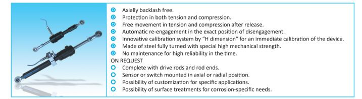
Safety coupling with linear limitation of force. Releasing both in compressive and tension once it reaches the calibration force. The setting force can be adjusted by turning the adjuster nut onto the springs and re-engagement is automatic. Possibility of connecting linear motion also very distant from each other.
